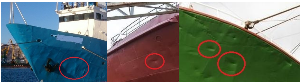
Fig. 1 – Typical minor damage of the ship's surface
