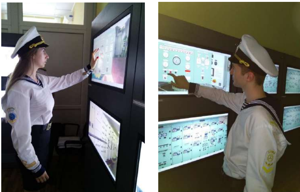
Figure 1. Participants in the non-immersive VR engine room simulator preparing Ro-Pax ferry emergency generator to the start (on the left); Starting process of the tanker LCC emergency generator (on the right)
